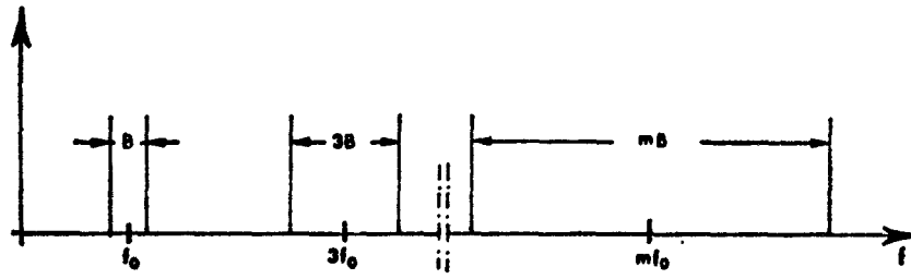
Fig. 3. Spectral band distribution of a phase-sampled waveform.
